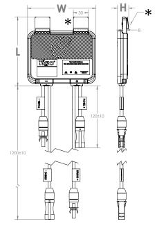
\*Clips can be removed for rack mounting
